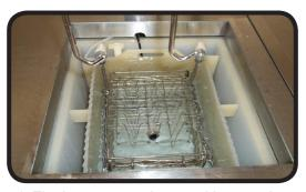
The lenses are submerged into an ultrasonic washing station. The water is purified to remove all trace minerals. When they are removed, the surface is free from water spots and imperfections.
