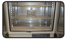
8. Finally, the lenses are thermally cured in a special oven for 2 hours. If you choose, AR or mirror coatings can be added at this point.
