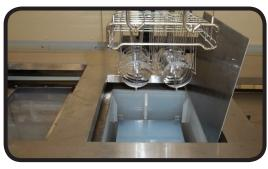
The lenses are then transported to the primer bath where they receive a light coating of an adhesion material. This ensures the scratch coating will form a bond with any lens material.
