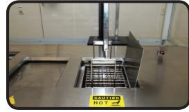
4. Once the primer base coat is applied, the lenses are moved to a small thermal curing station. This allows the primer to bond successfully with the scratch coating solution.
