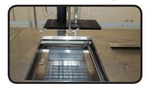
The lenses stay immersed in the scratch coating solution for a full 5 minutes.
