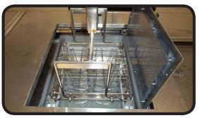
5. Much like the primer step, the lenses are slowly lowered into the scratch coating solution.
