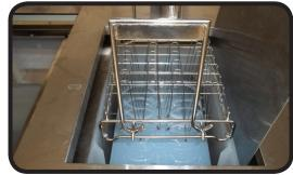
3. The robotic arm slowly lowers the lenses into the primer base coat solution. This slow insertion and removal guarantees a lens free from runs and drips.
